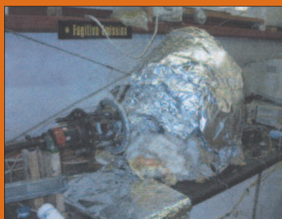
Fig. 2b: During the test, the valve is insulated.
