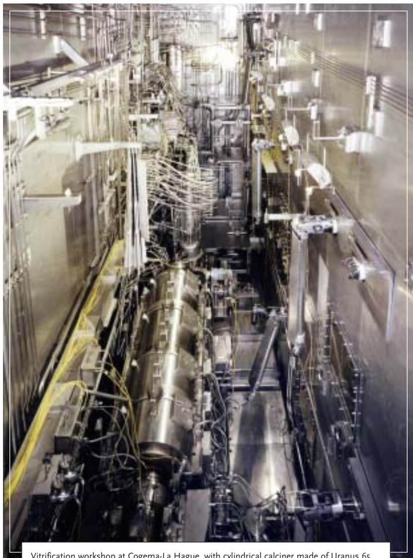
Vitrification workshop at Cogema-La Hague, with cylindrical calciner made of Uranus 65
