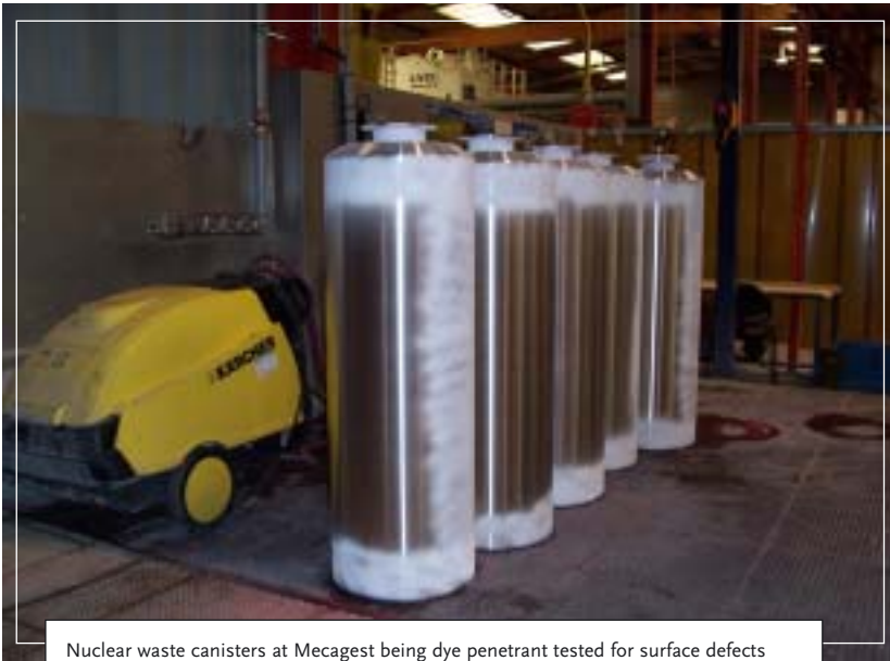
Nuclear waste canisters at Mecagest being dye penetrant tested for surface defects
