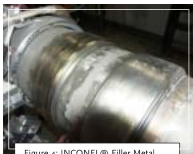
Figure 4: INCONEL® Filler Metal 52M (ERNiCrFe-7a) structural weld overlays
