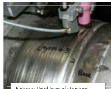
Figure 3: Third layer of structural weld overlay
