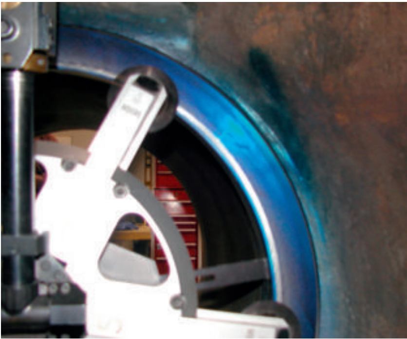
Three degree angle grinding on the outside diameter of an in-body valve seat.
